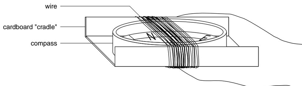
3. When you finish wrapping, leave 21 cm of free wire on the other end also. Twist the free ends together near the cradle a few times to keep the coil from unraveling.
