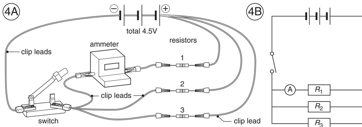
Circuit with ammeter connected between the switch and resistor 1: wiring diagram (A) and circuit diagram (B)
