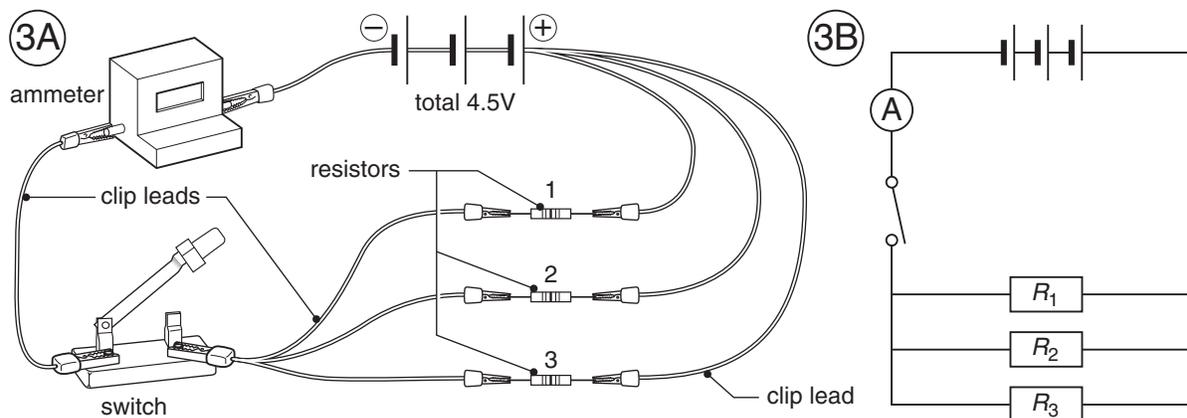
Circuit with ammeter connected between the switch and a cell: wiring diagram (A) and circuit diagram (B)
