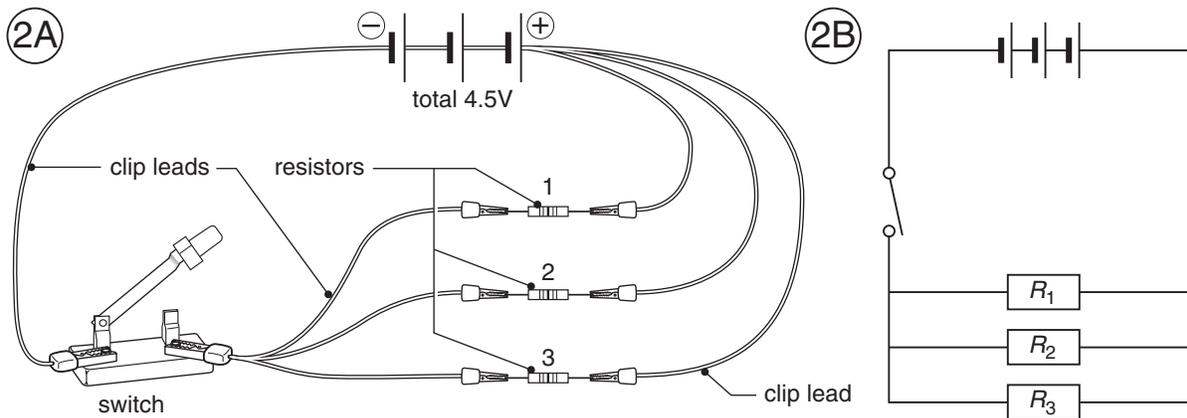
Circuit with three resistors connected in parallel: wiring diagram (A) and circuit diagram (B)
