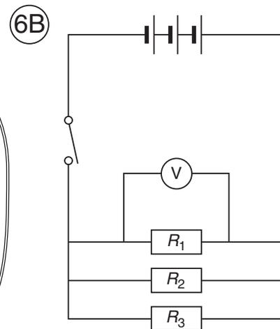
Voltmeter connected to measure voltage across resistor 1: wiring diagram (A) and circuit diagram (B)
