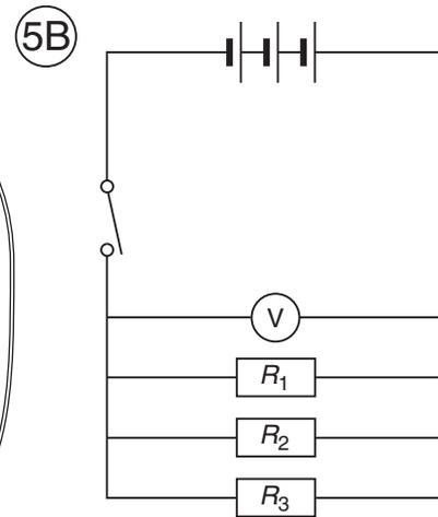
Voltmeter connected to measure voltage across all three resistors: wiring diagram (A) and circuit diagram (B)
