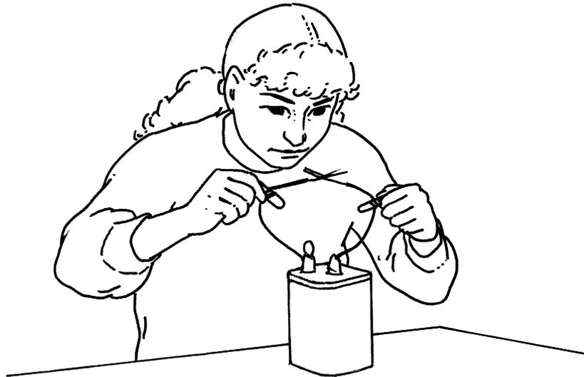
5. **Test** whether an object is a conductor or an insulator by touching both wires to the object. See if the bulb lights. **Record** your observations in the data table.
